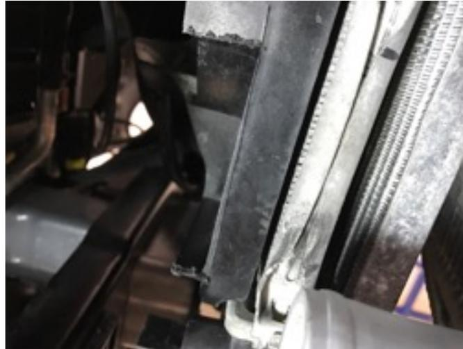
Now to remove a portion of the vertical side of the shroud, use the hacksaw blade to cut into the shroud about three inches up from the bottom, as shown in the photo, and once again score a deep cut from the cut you just made with the hacksaw to the bottom of the shroud as shown in photo below.
