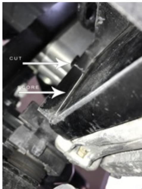
Once complete use a pair of needle nose pliers to break away the remaining piece.
