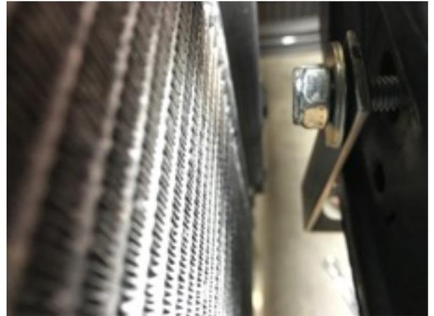
Do not tighten down the nuts, just get them on until you feel the resistance from the nylon lock nut.
