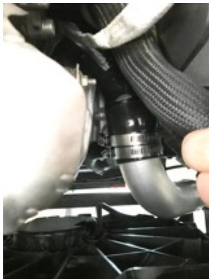
Next position the bottom portion of the charge pipe in the area between the frame and the modified fan shroud, and install the ninety degree silicone hose.
