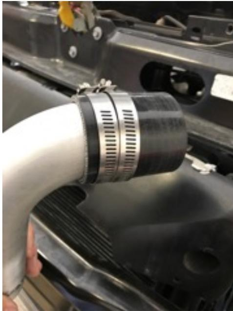
Next drop the charge pipe into position from above, through the engine compartment.
