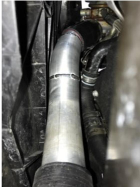
Once hose is on turbo outlet, slide up the clamp and secure it in position.
